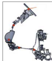
Energy absorbing type steering column
